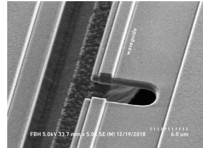
Fig. 2. Intermittent wave guide section to allow for interaction between Rydberg atoms and light.
