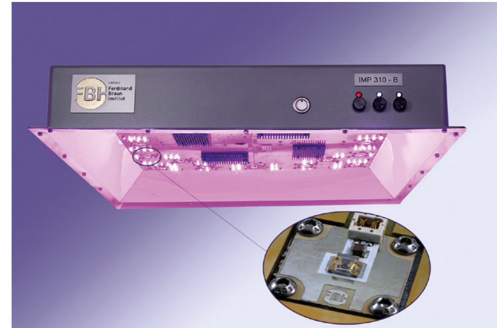
Fig. 3: Irradiation module for plant growth investigations consisting of UVB LEDs (310 nm) combined with red (660 nm) and blue (451 nm) LEDs.
