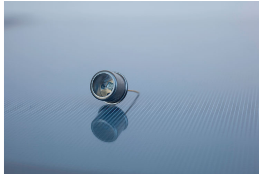
Fig. 1. Packaged UV photodiode. The edge length of the square chip is 1 mm.
