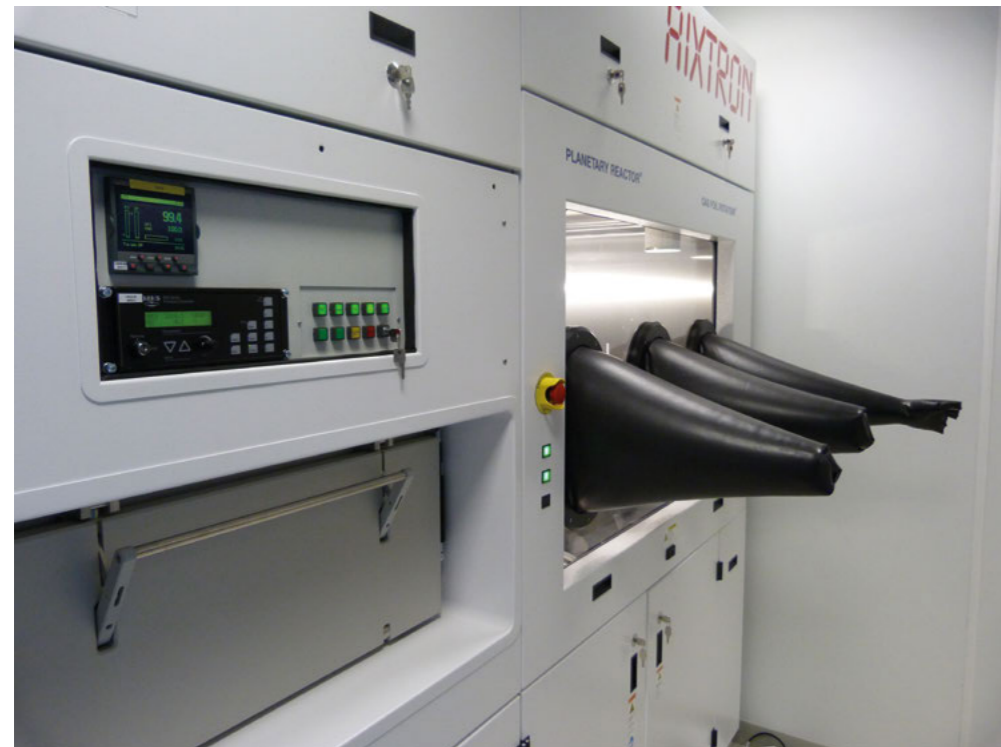
12x4" MOVPE reactor for GaAs-based layer structures.
